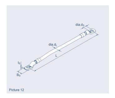
Table 8: Dimensions of the Earthing Connectors Type 71 EV S95
