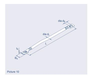
Table 7: Dimensions of the Earthing Connectors Type 71 EV K50 / K70
