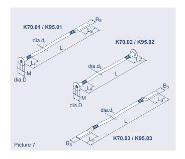
Table 5: Dimensions of the Earthing Sleeve Type 71 EB K70 / K95
