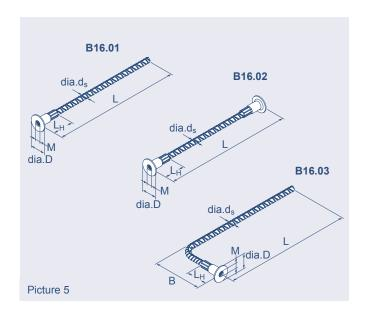
Table 4: Dimensions of the Earthing Sleeve Type 71 EB B16
