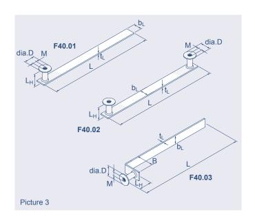
Table 3: Dimensions of the Earthing Sleeve Type 71 EB F40
