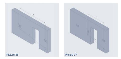
Every planning of anchoring must fundamentally adhere to the "n" and "f" dimensions. The maximum distances are indicated in table 19 on page 17 and in tables 21 + 22 on page 20.
