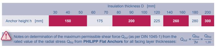
All rating values for shear force  $Q_{Rd}$  [kN] presented here for **PHILIPP Flat Anchors** apply to buildings of heights  $\leq$  100 m and a minimal concrete quality of C30/37 (fck, <sub>cyl</sub> = 30 N/mm<sup>2</sup>, fck, <sub>cube</sub> = 37 N/mm<sup>2</sup>) based on DIN 1045-1
